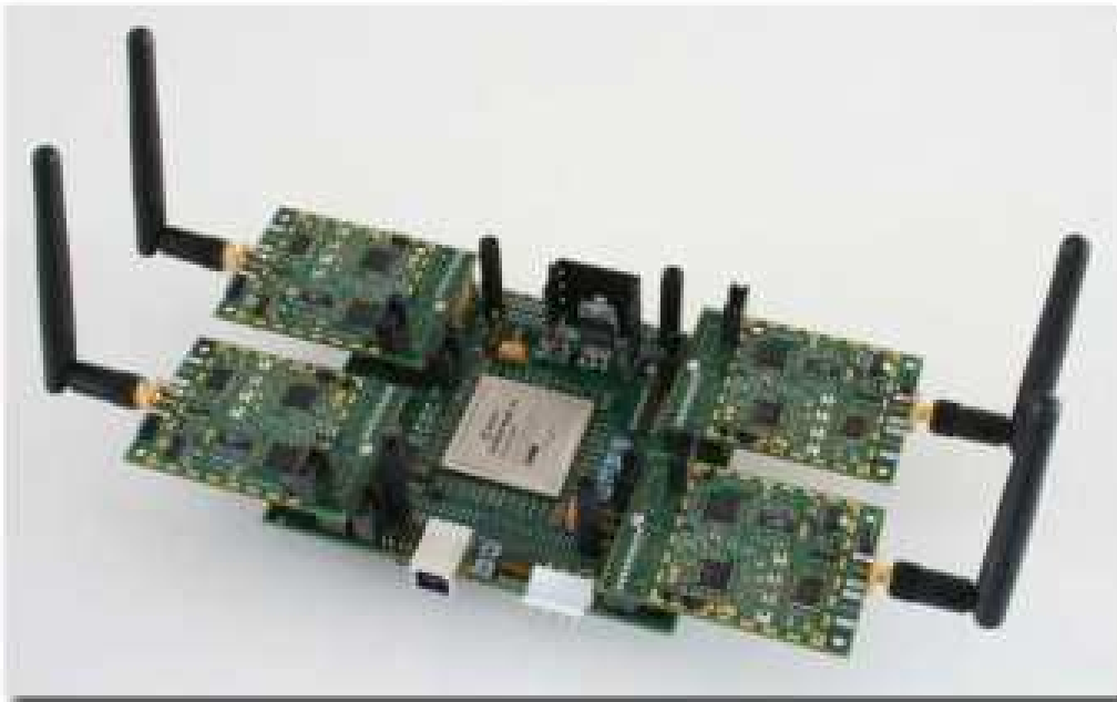
Figure 2.6: Picture of the integrated MIMO-RF with additional baseband FPGA carrier (QuadBAT platform) [2]
