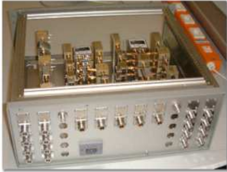
Figure 2.3: Picture of the RF box, built from discrete RF components, used in the ETHZ MIMO-OFDM testbed
